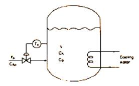
Q2. An isothermal, irreversible reaction  $A \xrightarrow{k} B$  takes place in the liquid phase in a constant volume reactor. The mixing is not perfect. Observation of flow pattern indicates that a two tank system with back mixing as shown in Figure. Assuming FR are constant, write the equations describing the system.
